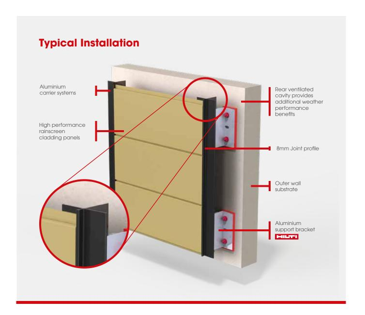
The Eltherington EPS uses 2mm extruded aluminium that allows for a quick, simple and secret fix install. The standard plank returns along with our extruded vertical profile ensures an accurate 8mm vertical and horizontal joint gap.
